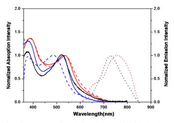
**Fig. 1.** Absorption spectra of **JK-91** (red solid line), **JK-92** (blue solid line) and **N719** (block solid line) in DMF, together with the absorption spectra of **JK-91** (red dash line) and **JK-92** (blue dash line) adsorbed on TiO<sub>2</sub> film and their emission spectra of **JK-91** (red dot line) and **JK-92** (blue dot line). (For interpretation of the references to colour in this figure legend, the reader is referred to the web version of this article.)
