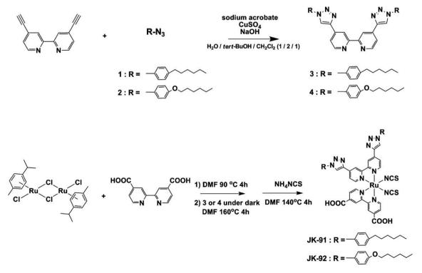
Scheme 1. Schematic diagram for the synthesis of ruthenium sensitizers 5 and 6.
