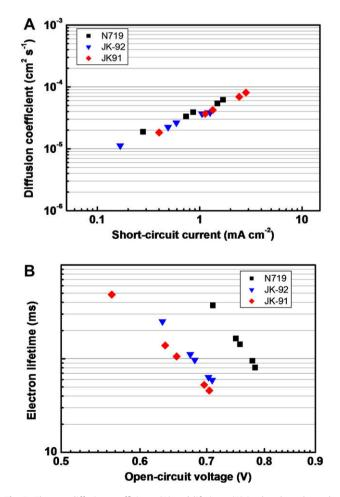
Fig. 5. Electron diffusion coefficients (A) and lifetimes (B) in the photoelectrodes adsorbing different dyes (i.e., JK-91, JK-92 and N719).
