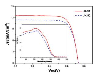
**Fig. 4.** I–V curves and IPCE spectra for **JK-91** (red solid line) and **JK-92** (blue dash line). (For interpretation of the references to colour in this figure legend, the reader is referred to the web version of this article.)
