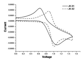
Fig. 2. CV of JK-91 (solid line) and JK-92 (dash line) on TiO<sub>2</sub> film with 0.1 M (n-C<sub>4</sub>H<sub>9</sub>)<sub>4</sub>NPF<sub>6</sub> acetonitrile solution (scan rate of 50 mV s<sup>-1</sup>).
